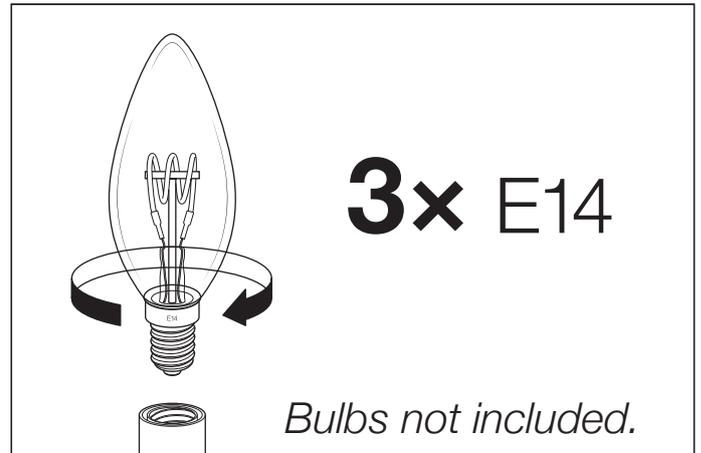
4. Carefully place the bulbs in the fittings. Do NOT turn the bulbs further than necessary, to prevent damage to the fitting.
