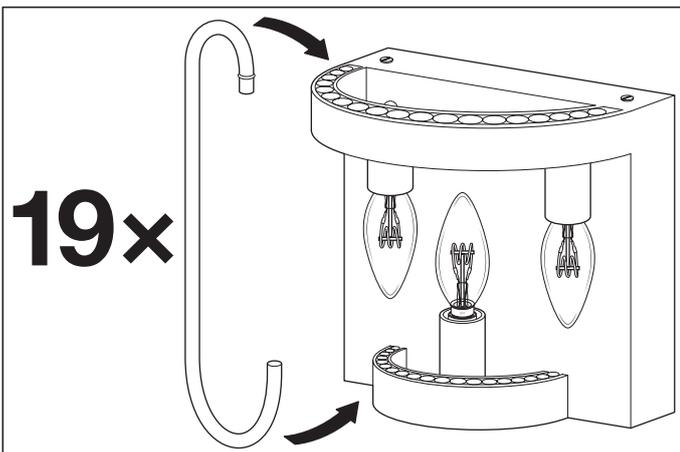
5. Carefully place the glass rods inside the holes on the frame. First place the bottom of the rod inside the hole, then the top side of the rod.
