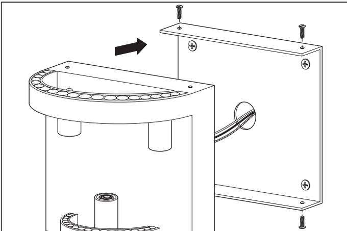
3. Carefully place the lamp over the wall plate and align the holes in the wall plate with the holes in the lamp. Secure the screws on all sides.
