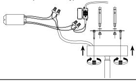
**5** Connect the 3 power wires with the transformer according to their colours. Brown is the live wire, blue is the neutral wire, green/yellow is the earth wire. Place the ceiling canopy flush against the ceiling and fix it securely with the two nuts supplied.
