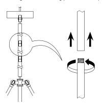
**2** Place the middle rod upright and fix the three pipes with the wing nuts on top and bottom side.
